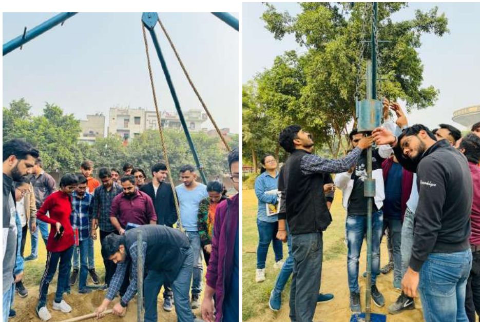
Glimpse of Soil Testing using SPT
