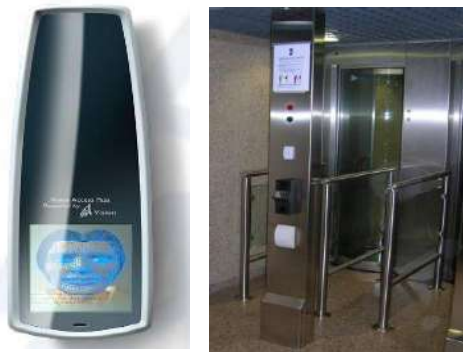
New face reader with LCD Access control into banks
