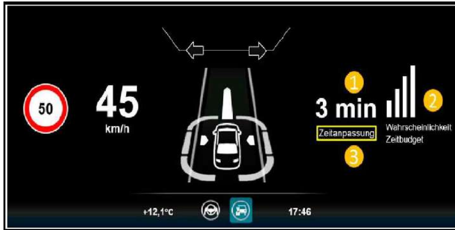
Figure 3 is a design of a HMI that notifies the operator of the rationale for an urgent maneuver's activation.
