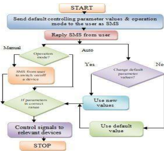
Fig. 6: Flowchart of the program for the proposed system
