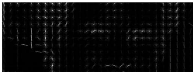
The original image is turned into a HOG representation that captures the major features of the image
