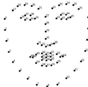
The 68 landmarks we will locate on every face. This image was created by Brandon Amos of CMU who works on OpenFace.
