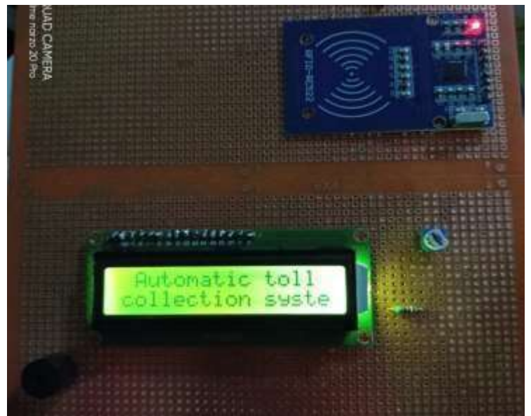
Fig. 5: Automatic Toll System.
