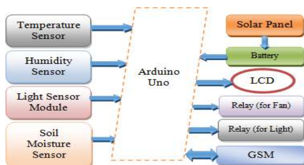
Fig. 1: Block Diagram of Greenhouse Monitoring System
